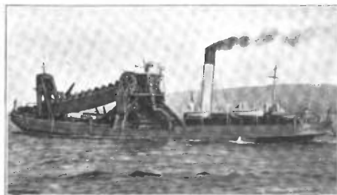
Fig. 10.—Hopper-dredger, "David Dale," with buckets of 54 cub. ft. capacity (see fig. 11) built for the North Eastern Railway Company by Lobnitz & Co.
