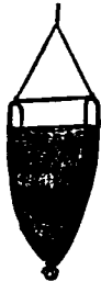
From Alexander E. Agassiz's Three Cruises of the "Blain" . By permission of Houghton, Mifflin & Co. FIG. 18.—Agassiz or Blake Trawl.
